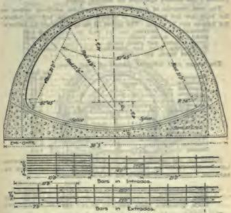
Fig. 23.—Reinforced Concrete Sewer.
